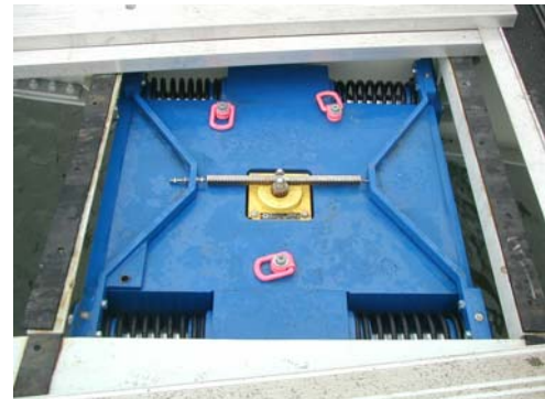
Fig. 10 Horizontal damping device
